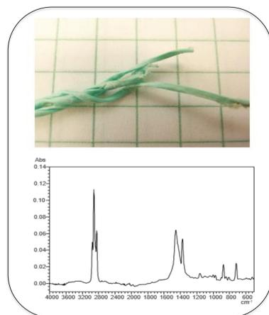
Figure 3: FTIR spectrum of fishing nets identified as Polyethylene/ Polypropylene
