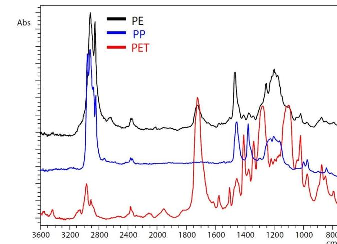
Figure 6: Typical Infrared Spectra from Areas in Figs.4-(a) to (c)
