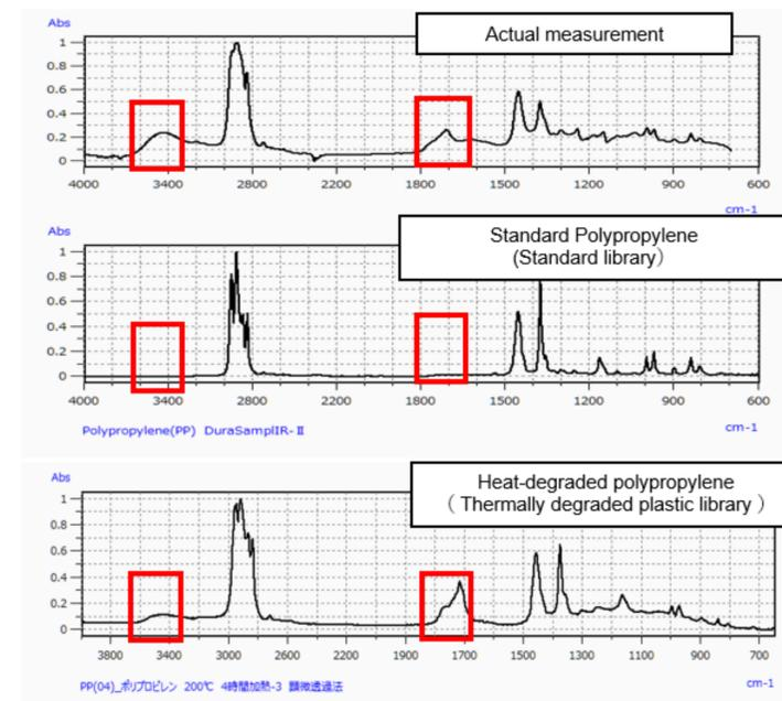
Figure 4: Infrared spectrum and library search result of MPs
