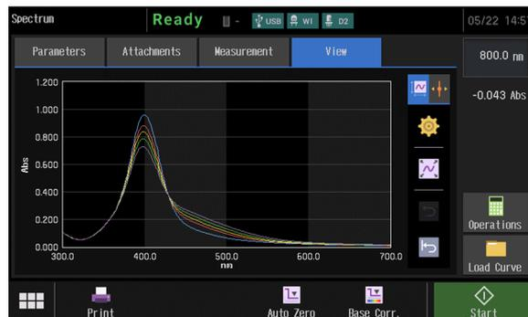
**Fig. 6 Absorption Spectra of 30 nm Silver Nanoparticles Aqueous Solution After Adding NaCl Aqueous Solution From the top, 0 seconds, 30 seconds, 1 minute, 2 minutes and 4 minutes after adding NaCl solution**
