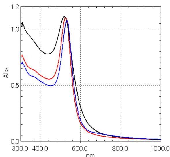
Fig. 2 Absorption Spectra of Gold Nanoparticles with different particle size
