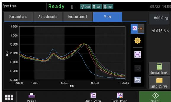
**Fig. 4 Absorption Spectra of 30 nm Gold Nanoparticles Aqueous Solution After Adding NaCl Aqueous Solution From the top, 0 seconds, 30 seconds, 1 minute, 2 minutes and 4 minutes after adding NaCl solution**
