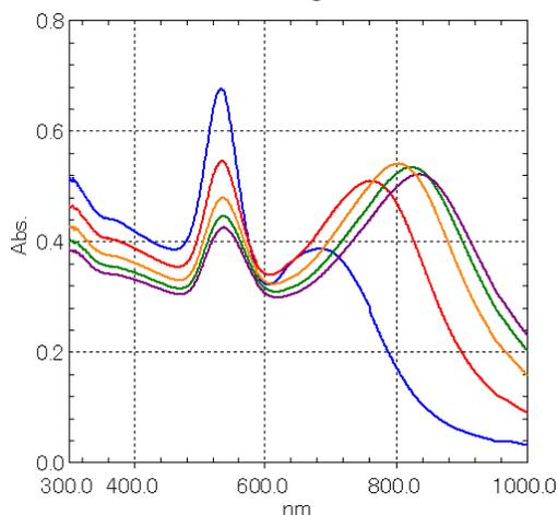
**Fig. 5 Absorption Spectra of 50 nm Gold Nanoparticles Aqueous Solution After Adding NaCl Aqueous Solution Black: 0 seconds, Red: 30 seconds, Blue: 2 minutes, Green: 5 minutes, Purple: 10 minutes after adding a NaCl solution**
