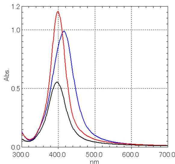
Fig. 3 Absorption Spectra of Silver Nanoparticles with different particle size
