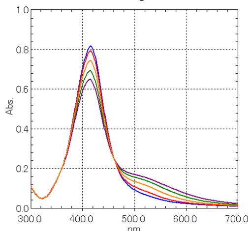
**Fig. 7 Absorption Spectra of 50 nm Silver Nanoparticles Aqueous Solution After Adding NaCl Aqueous Solution Black: 0 seconds, Red: 30 seconds, Blue: 2 minutes, Green: 5 minutes, Purple: 10 minutes after adding a NaCl solution**
