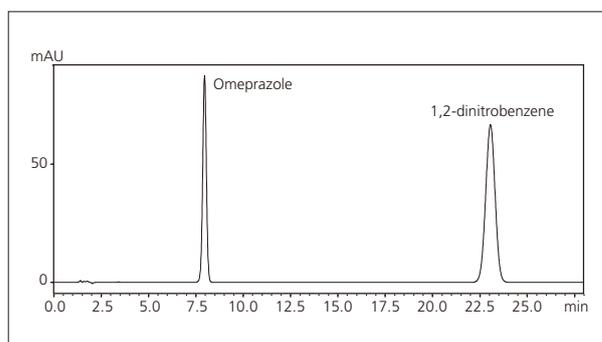
**Fig. 3 Chromatogram According to JP Method – System Performance**
