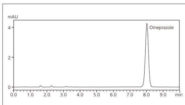
**Fig. 4 Chromatogram According to JP Method – System Repeatability**
